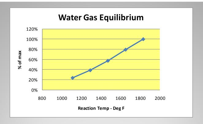
Optimum Reaction Temperature is between 1600 and 1800 F
