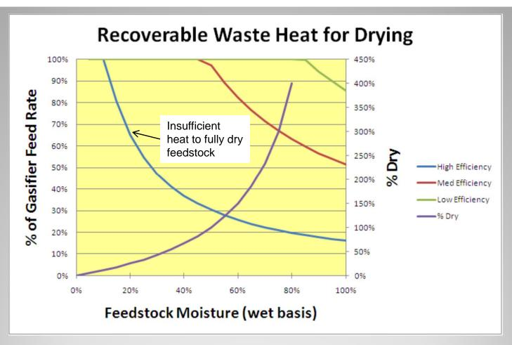
High efficiency gasifiers (high calorific value gas) do not have sufficient recoverable waste heat for adequate feedstock drying.
